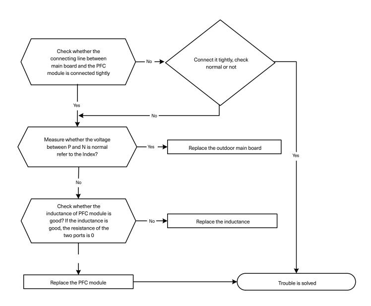
TS31: Communication error between outdoor main chip and compressor driven chip diagnosis and solution
