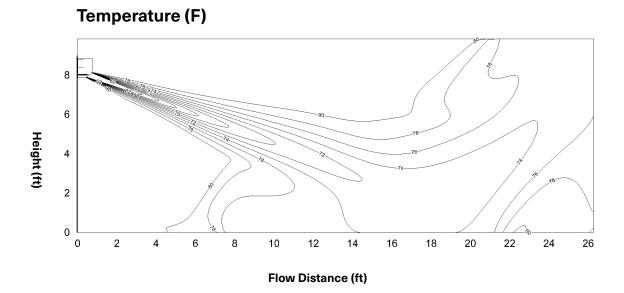
24k-Heating (ID: 20°C/68°F, OD: 7°C/44.6°F) Discharge Angle 77°
