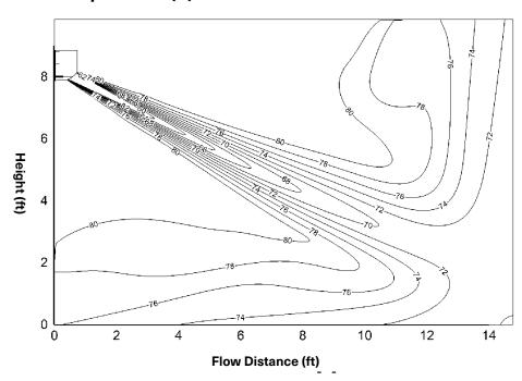
12k-Heating (ID: 20°C/68°F, OD: 7°C/44.6°F) Discharge Angle 90°
