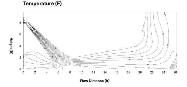
36k-Cooling (ID: 27°C/80.6°F, OD: 35°C/95°F) Discharge Angle 55°
