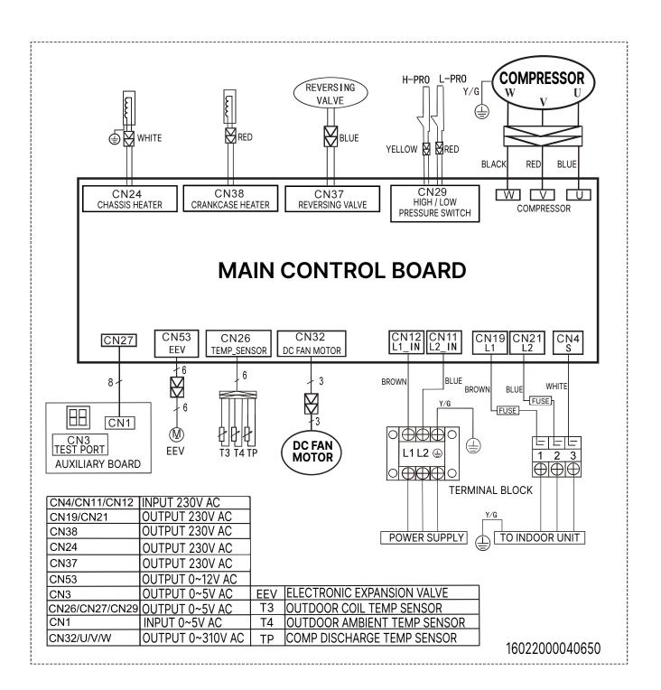
Outdoor unit printed circuit board diagram: 17122000062141
