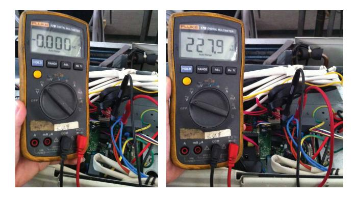
1. Turn off the power, use a digital tester to measure the resistance. The value should be  $1.8 \sim 2.5 \text{ K}\Omega$ .
