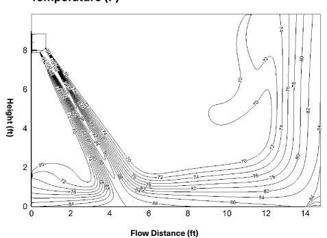
18k-Cooling (ID: 27°C/80.6°F, OD: 35°C/95°F) Discharge Angle 50°
