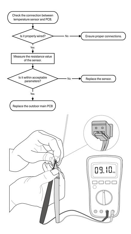
Note: For certain models, outdoor unit uses combination sensor, T3, T4 and TP are the same of sensor. This picture and the value are only for reference, actual appearance and value may vary.
