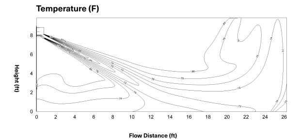
36k-Heating (ID: 20°C/68°F, OD: 7°C/44.6°F) Discharge Angle 75°
