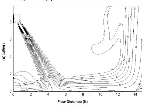
9k-Cooling (ID: 27°C/80.6°F, OD: 35°C/95°F) Discharge Angle 58°
