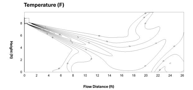
18k-Heating (ID: 20°C/68°F, OD: 7°C/44.6°F) Discharge Angle 84°
