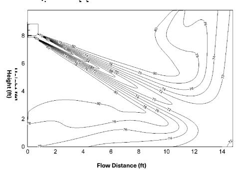
9k-Heating (ID: 20°C/68°F, OD: 7°C/44.6°F) Discharge Angle 90°
