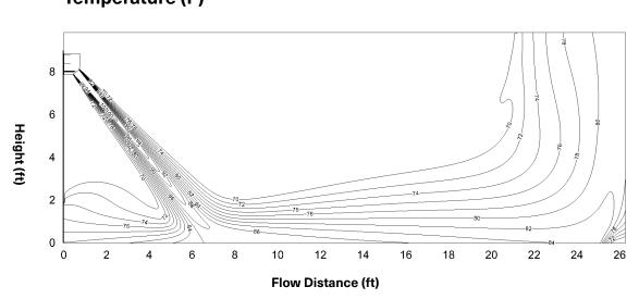
30k/33k-Cooling (ID: 27°C/80.6°F, OD: 35°C/95°F) Discharge Angle 55°
