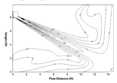
6k-Heating (ID: 20°C/68°F, OD: 7°C/44.6°F) Discharge Angle 90°
