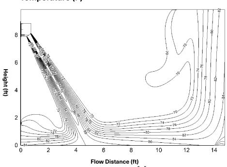
12k-Cooling (ID: 27°C/80.6°F, OD: 35°C/95°F) Discharge Angle 58°
